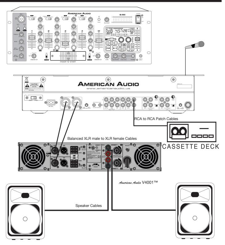
Typical Balanced Output Set-up
